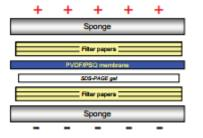
Left: a representation of the components of a transfer "sandwich". Notice the all-important orientation of the gel and membrane; of the two, make sure the PVDF membrane is situated nearest to the positive electrode. Amino acids are negatively charged and proteins will migrate in the direction of the positive charge.
