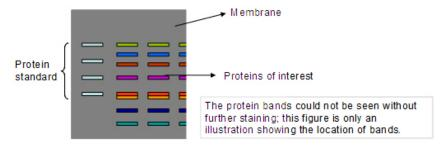
2. Detection Normally, secondary antibodies are conjugated to a reporter enzyme and the detection method used is based on the type of enzyme. The most commonly used enzyme for detection in western blotting is horseradish peroxidase (HRP), which reacts with its substrates to produce light. A photographic film is placed against the membrane and an image is created from the reaction.
